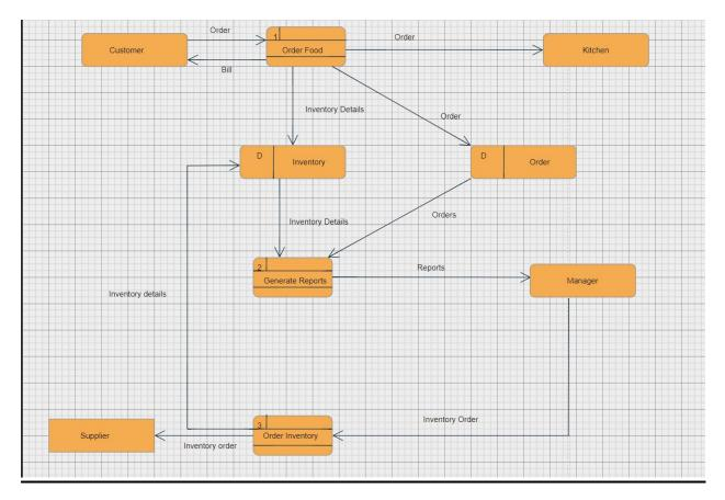
The Food Ordering System Data Flow Diagram contains three processes, four external entities and two data stores.
